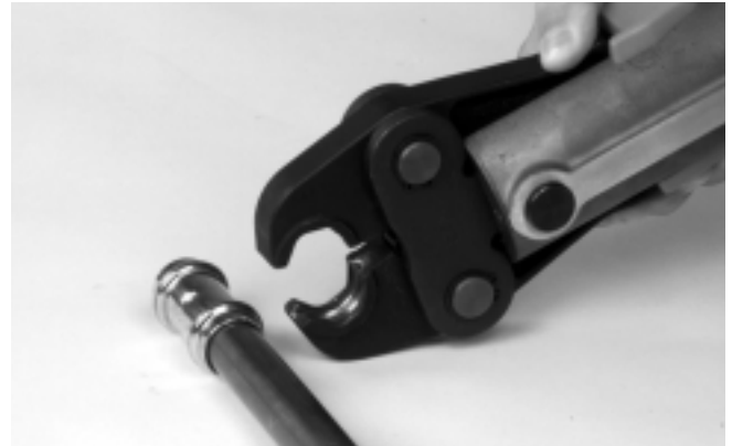
Figure 6 – Opening The SHP Jaw Set
