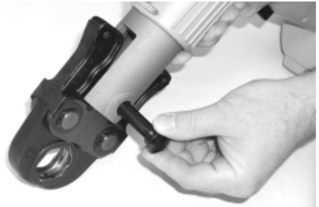
Figure 1 – Pulling The Jaw Set Mounting Pin Out
