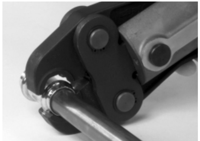
Figure 7 – Placing SHP Jaw Set Around Fitting
