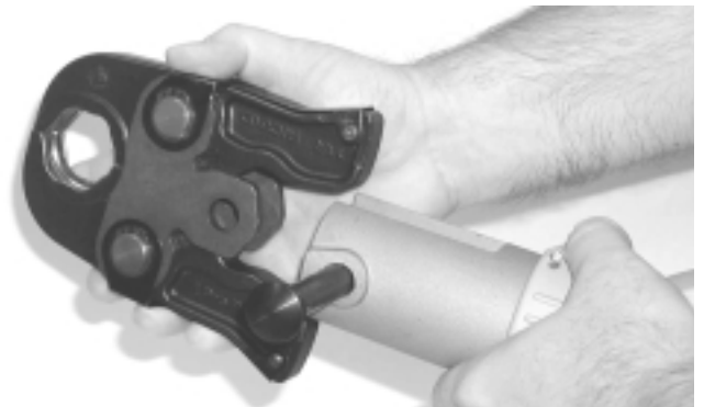
Figure 2 – Inserting Jaw Set
